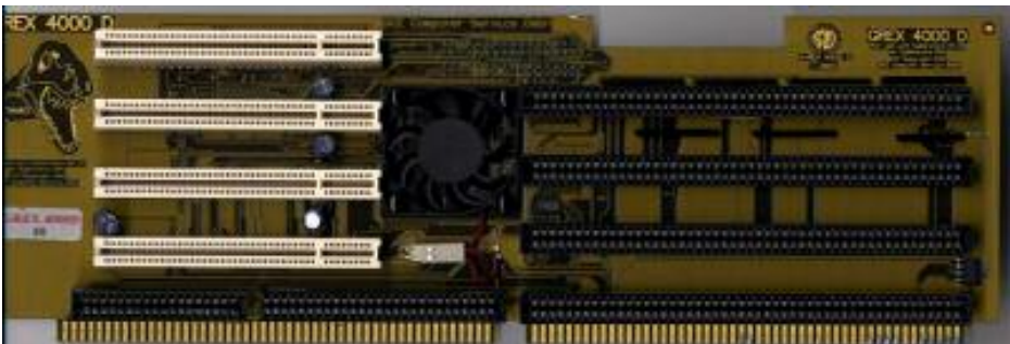
The G-REX 4000D card, fits perfectly on Every 4000, petty it needs a Blizzard PPC.
